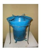
Conical shaped hopper with stand
